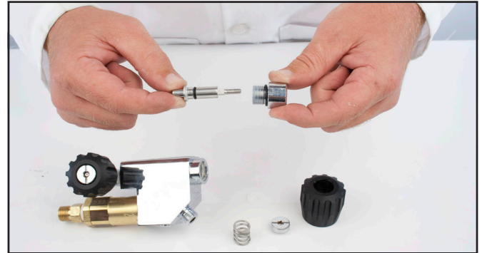
The valve stem usually comes out with the bonnet.
