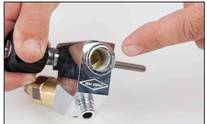
The seat should be removed for inspection.
