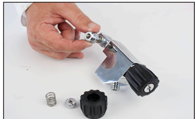
Installing the valve stem into the emergency valve.
