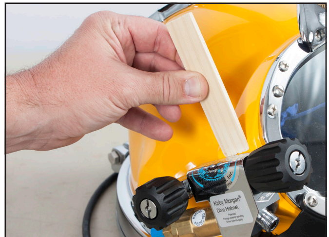
A wooden wedge helps to remove the side block.
