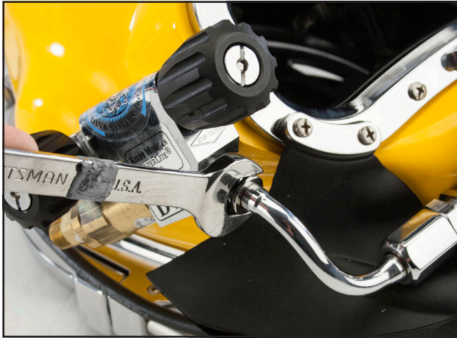
Loosening the bent tube from the side block.
