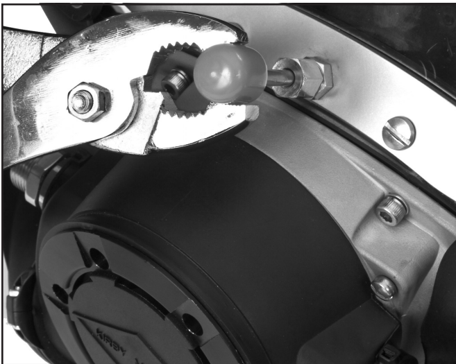
Protect the nose block device knob with a plastic cap or rag when you remove it.
