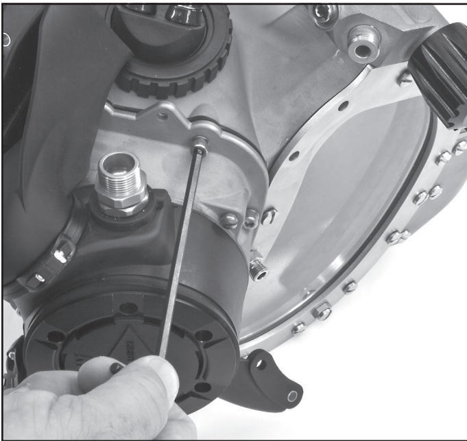
Tighten the nuts in a staggered pattern.
