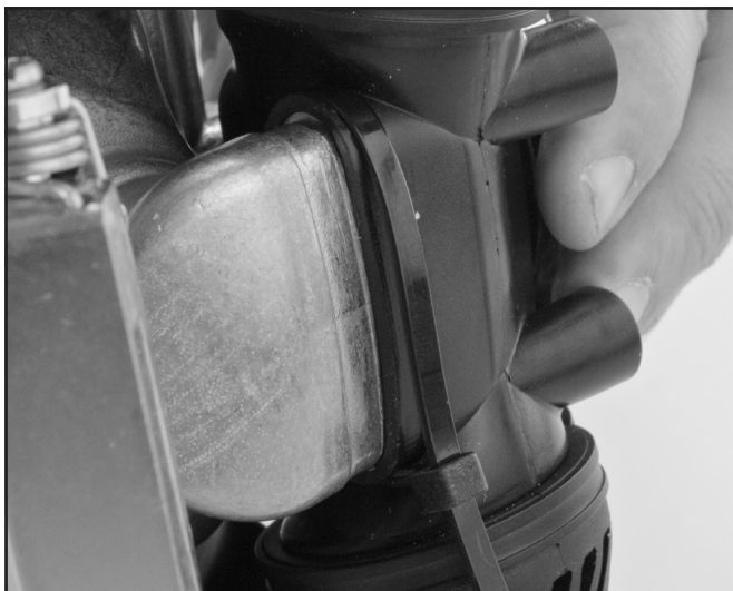
Insert the regulator into the pod.
