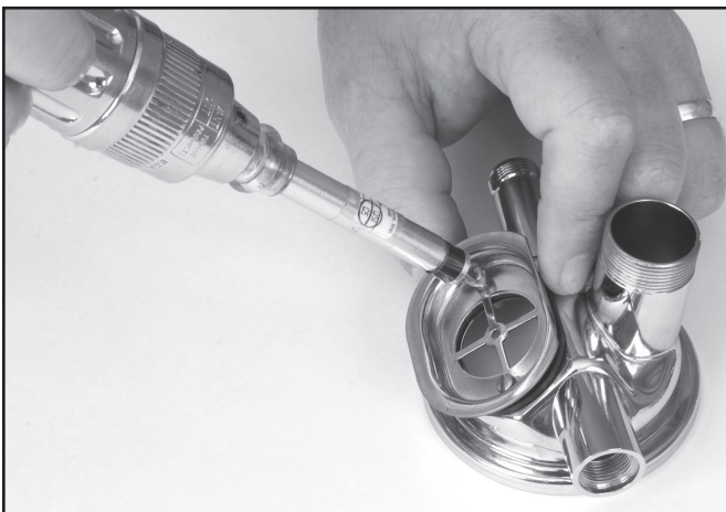
The screws that hold the flange on the regulator body should be tightened. See "Torque Specs" module.
