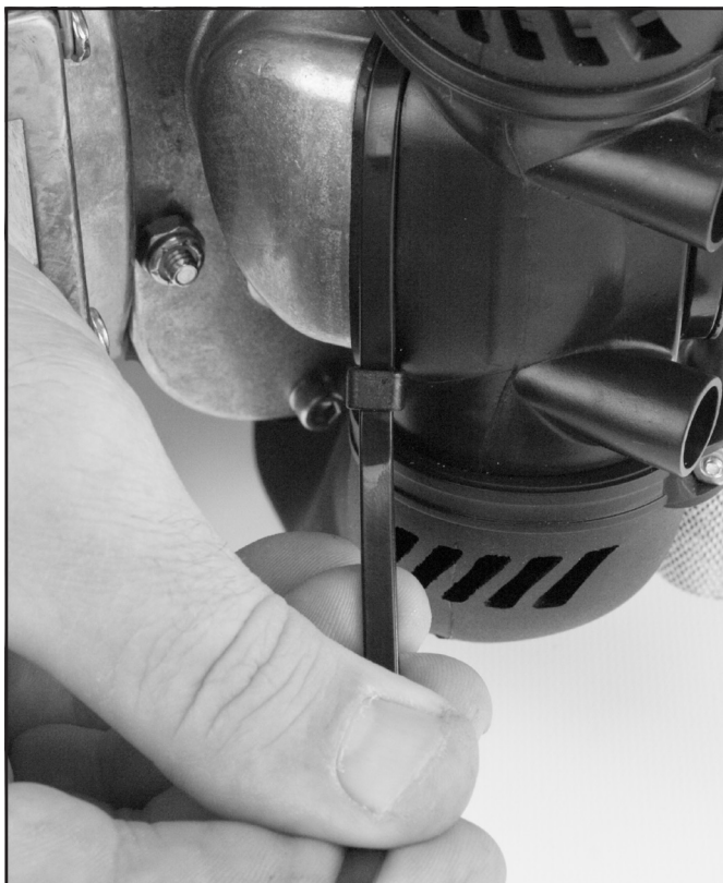
Carefully tighten tie wrap.
