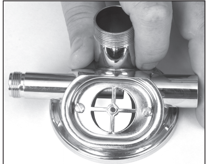
If the flange is tightened too much, the gasket will protrude into the exhaust valve opening and interfere with proper regulator performance.
