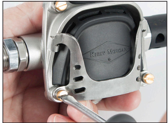
Install the diaphragm, cover assembly and cover retaining screws and torque.
