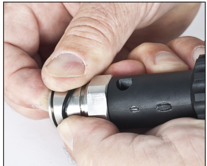
Remove the O-ring from the flex knob packing nut. You can use a credit card, toothpick, or any clean soft device that will not damage the O-ring or the nut.
