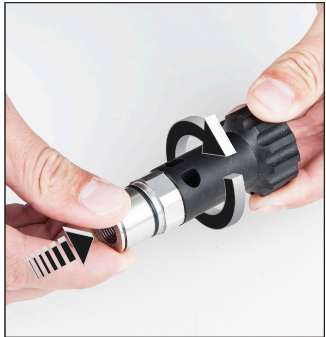
Push in on the adjustment shaft while turning the flex knob counterclockwise to engage threads
