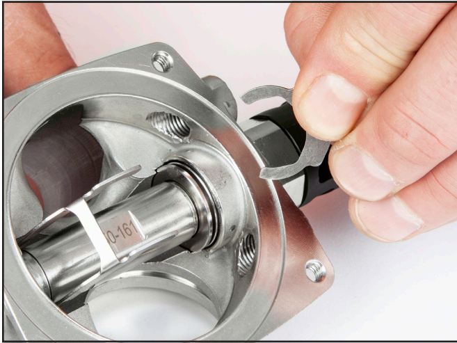
Install the lock clip on the main tube.
