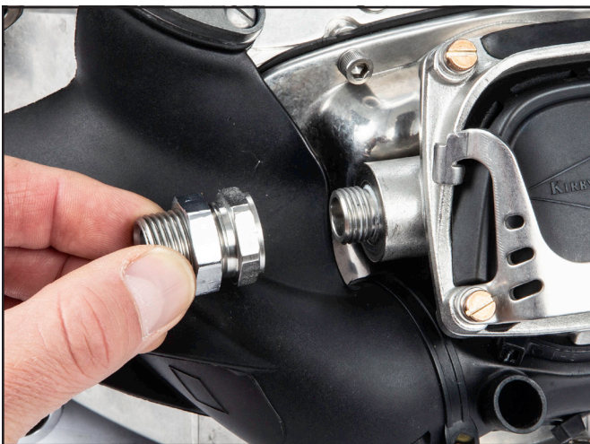
Remove the bent tube adapter.
