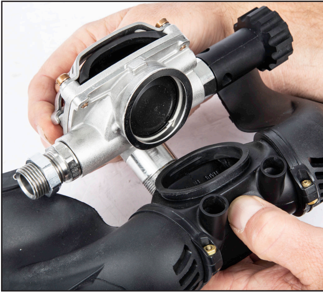
Install the main exhaust body onto the exhaust flange of the regulator body.
