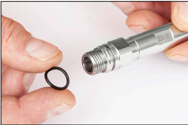
Install the O-ring onto the main tube.
