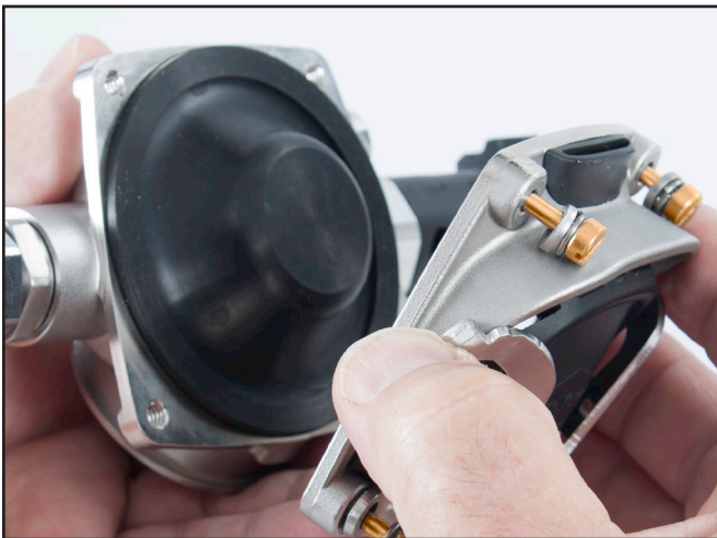
Fit the regulator cover retainer assembly onto the regulator body.
