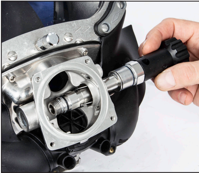
When you pull the flex knob assembly out, the main tube and related parts will follow.
