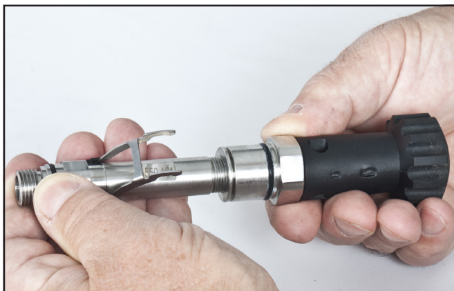
Unscrew the flex knob assembly from the main tube.
