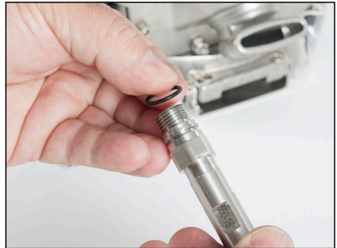
Remove the O-ring from the main tube.
