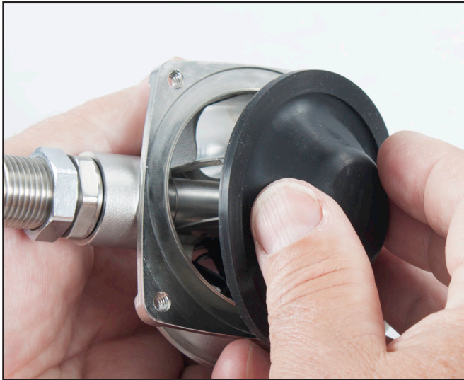
Place the diaphragm onto the regulator body.
