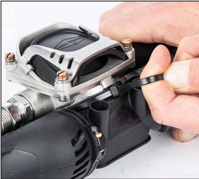
Install the tie wrap on the regulator.
