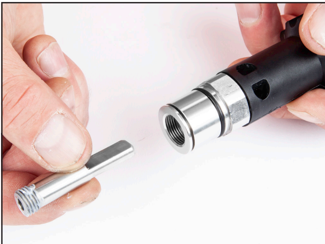
Lubricate the threads of the adjustment shaft with Christo-Lube® or equivalent and insert into the flex knob.
