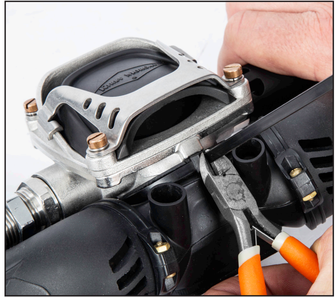
Remove excess tie wrap.
