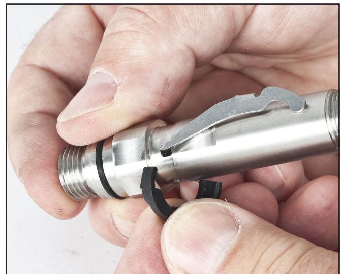
Remove the bearing clip.
