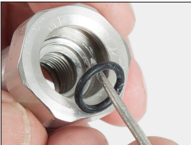
Using an O-ring pick, carefully remove the bearing washer and adjustment shaft O-ring.
