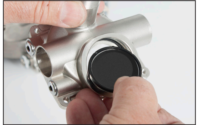
Install the O-ring and valve insert.
