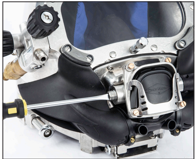
Turn the adjustment nipple \frac{1}{16} of a turn at a time to adjust the performance of the regulator.
