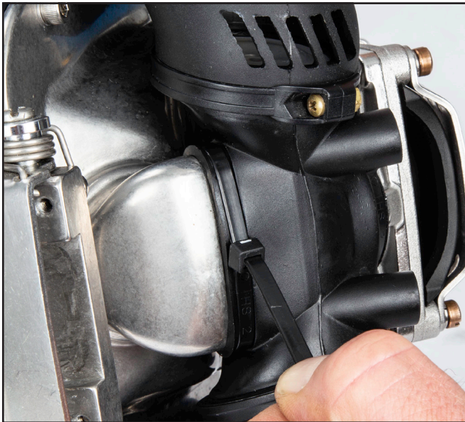
Secure and seal with a tie wrap.
