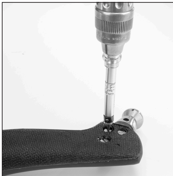
Begin the disassembly of the yoke by removing the latch catch assembly.
