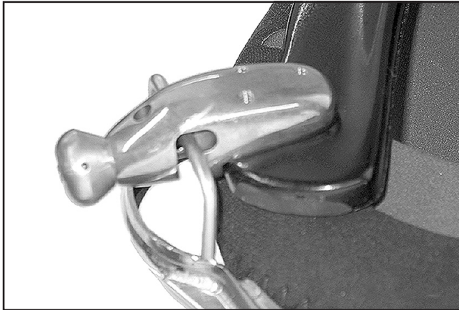
Proper adjustment of the neck clamp assembly should place the bail squarely in the groove of the latch catch body when the clamp is closed.
