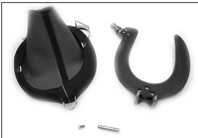
The yoke and neck clamp (with neck dam) must be separated from each other.
