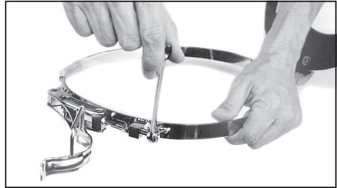
The neck clamp and latch catch must operate properly. They must be regularly inspected and serviced.
