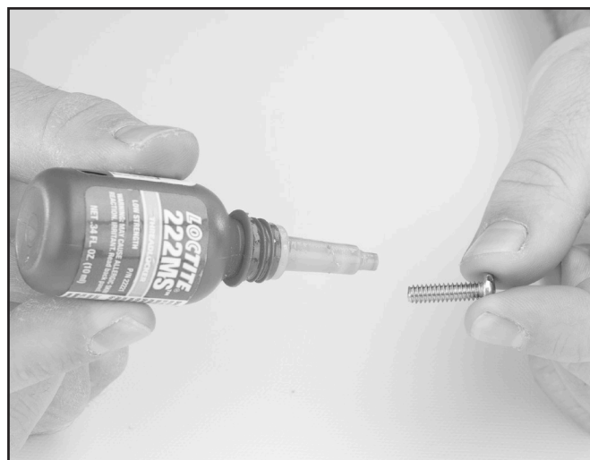
The latch catch assembly must be fastened to the yoke using Loctite® to secure the screws.
