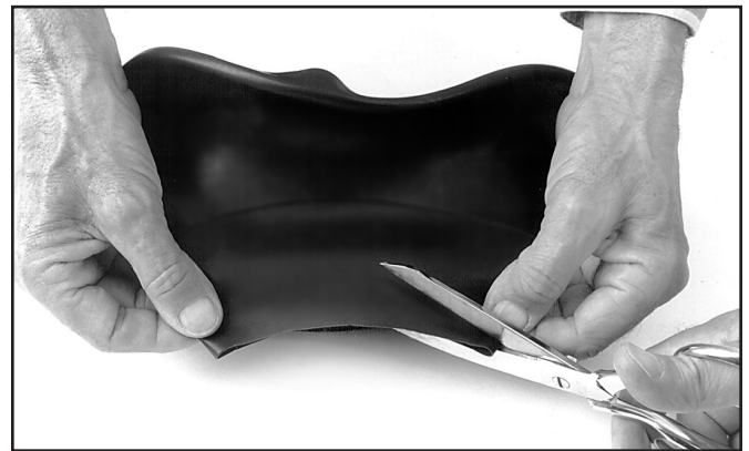
Trim latex neck dams with the largest, sharpest scissors available.
