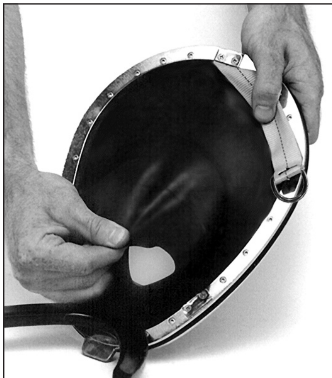
Check the neck dam for holes.
