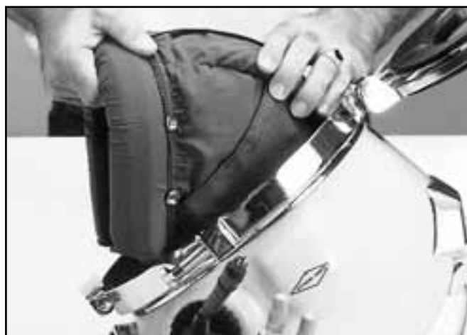
Removing the head cushion.
