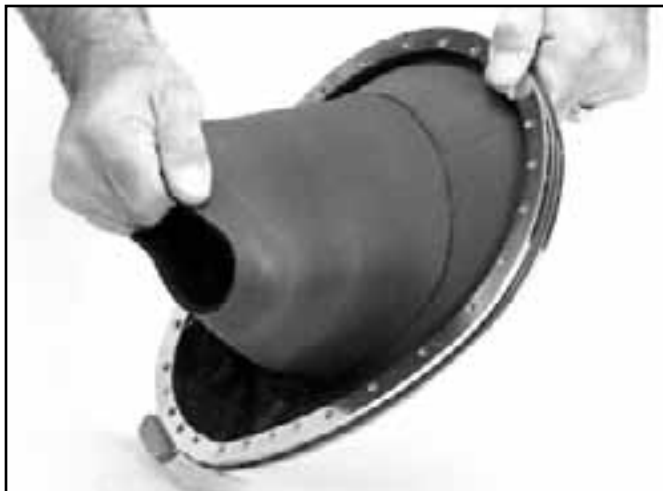
Check the neck dam for holes.
