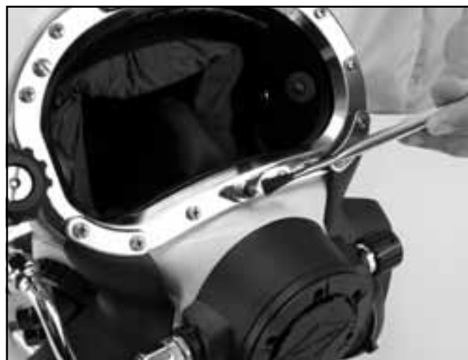
The nose block O-rings must be regularly lubricated.
