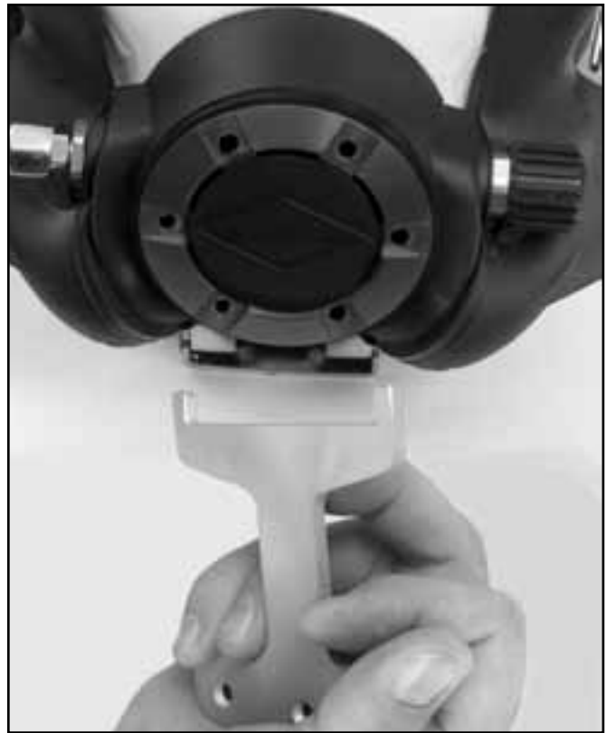
Remove the regulator cover to inspect the regulator exhaust valve.
