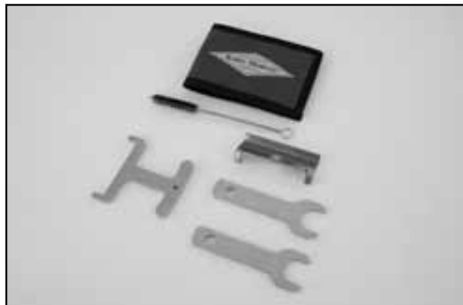
Special tools are required to do proper maintenance on the Kirby Morgan 47 helmet.
