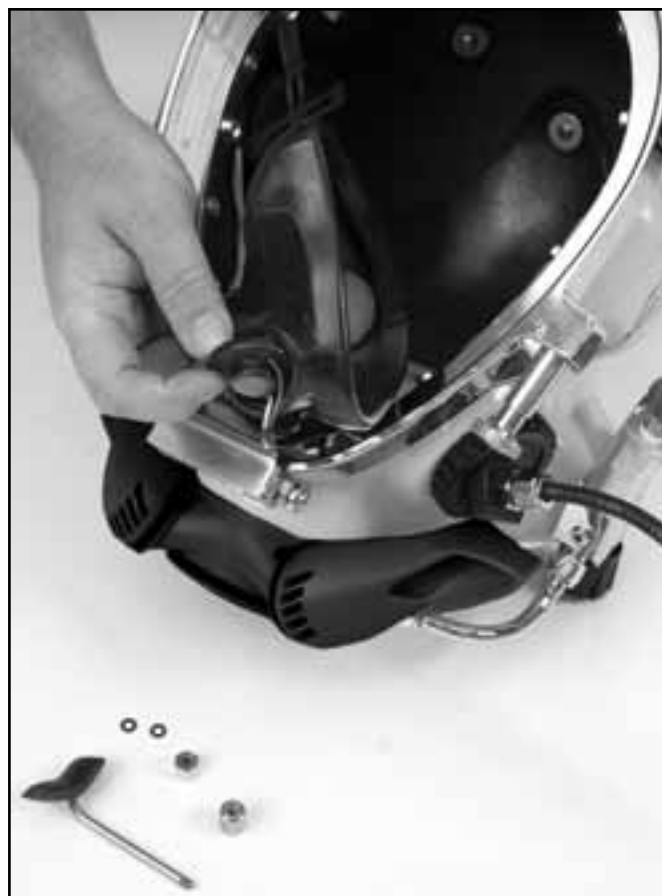
Remove the microphone so you can remove the oral/nasal mask.
