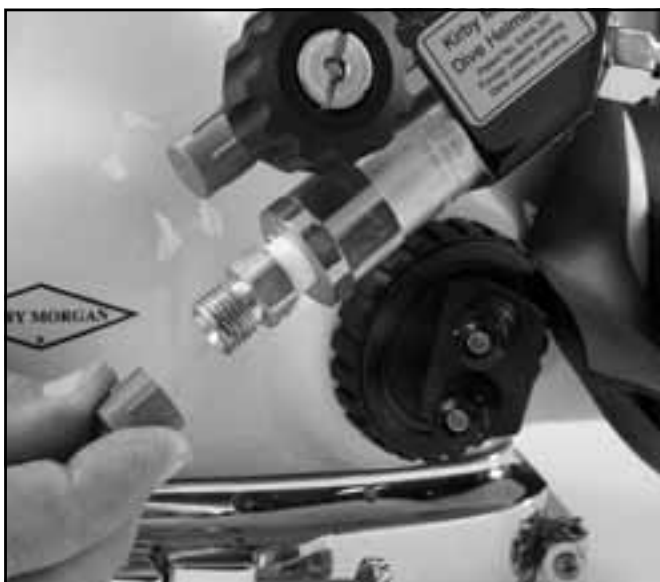
Cover the air inlet and emergency gas valve openings with dust caps when not in use.
