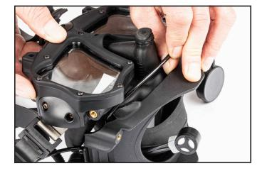
4) Bend the lens body away from the jaw frame and route the longer earphone wire across the front of the mask. Ensure the wire is pushed down into the gap found between these two parts of the mask. When the mask is released the wire should fit snugly into the groove.
