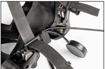
If the mask strap is installed, ensure the earphone wires are routed on the inside of the strap **NOT THE OUTSIDE**.
