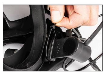
3) Use the included tie wrap P/N 520-038 to secure the communications assembly to the mask. Position the end or termination of the tie wrap so it won't be touching the diver's face.
