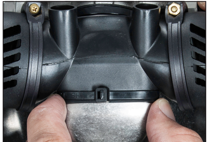
The Quad Valve must be properly connected to the regulator and the water dump cover on the pod.
