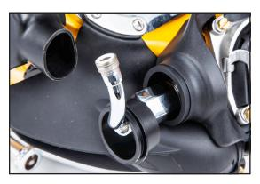
10) Swing the bent tube away from the side block and put the adapter sleeve (short), P/N 550-572, onto the bent tube assembly first, channeled end facing away from regulator inlet.
