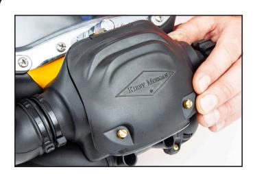
17) Close the access cover and secure by pushing over the bishop pins. Make sure the regulator shroud and access cover line up correctly and no part is pinched or tucked.
