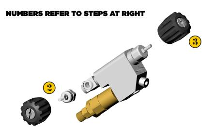
2) Remove the emergency valve control knob, screw, spring, washer, packing nut and stem.
