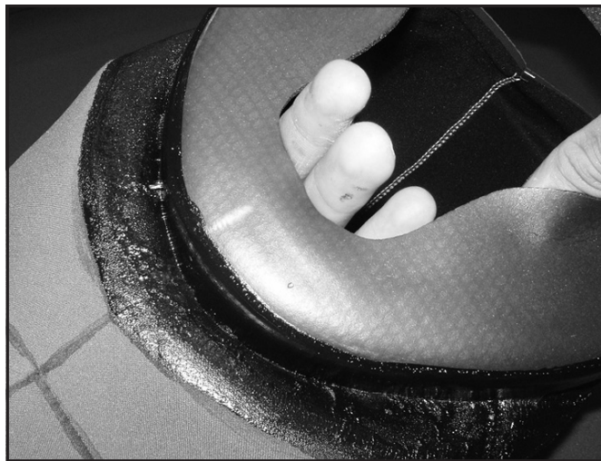
Start attaching the face seal to the hood at the bottom center of both.
