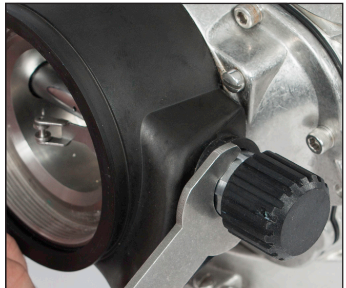
Tighten the packing nut on the adjustment knob.
