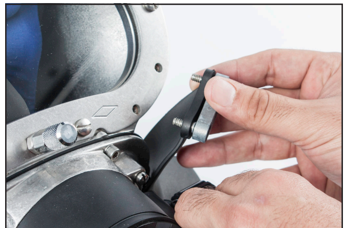
The whiskers are fastened to the face port using two screws on each side.
