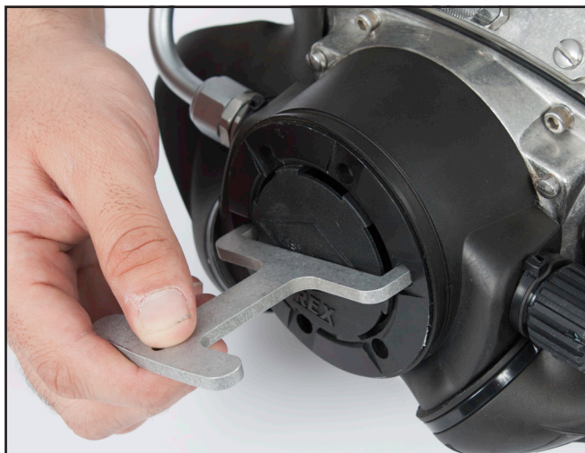
Start removal of the cover by unscrewing the retaining ring.
