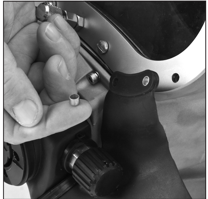
Make sure the whisker spacers are in position before tightening the screws that secure the whiskers.
