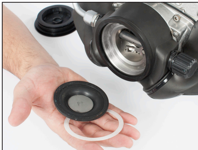
Remove the diaphragm and washer.
