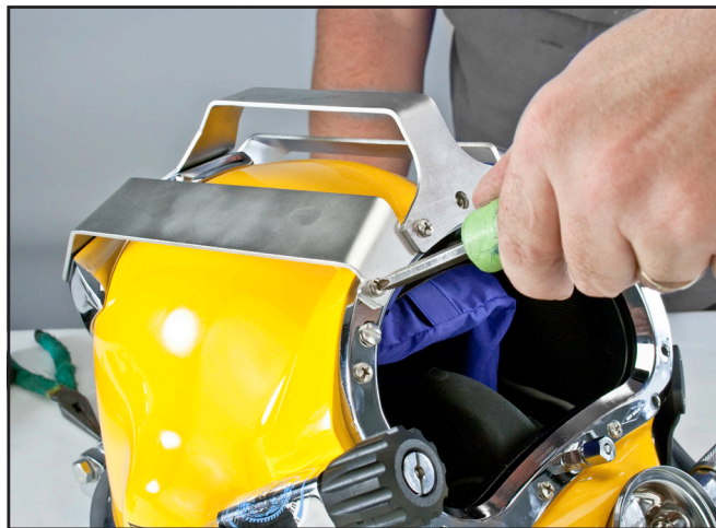
Remove the front mount screws
