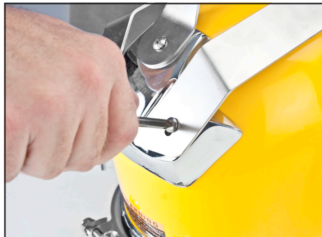
Remove the screw at the rear of the handle.
