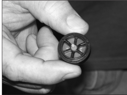
Figure 1: Installation of purge valve into purge valve body
