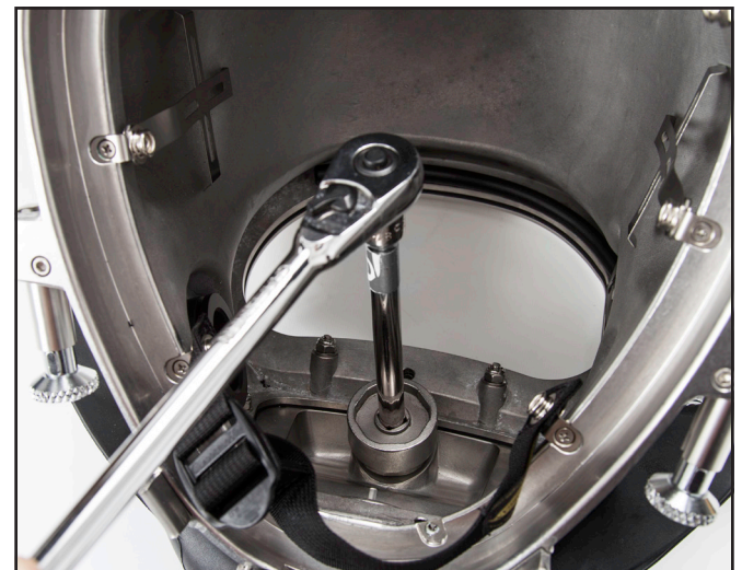
Removal of the regulator mount nut.
