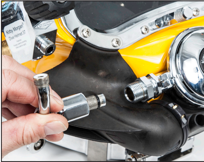
Removing the bent tube.
