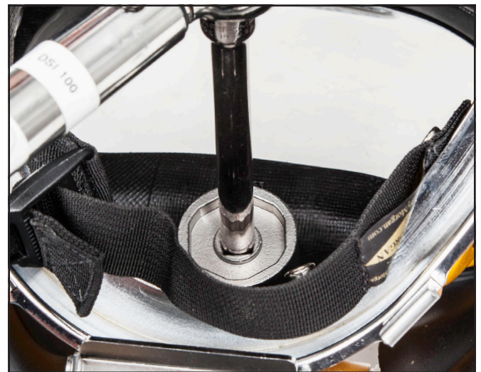
Removal of the regulator mount nut.
