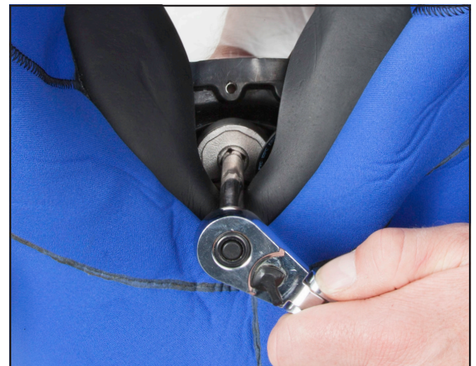
Removal of the regulator mount nut.
