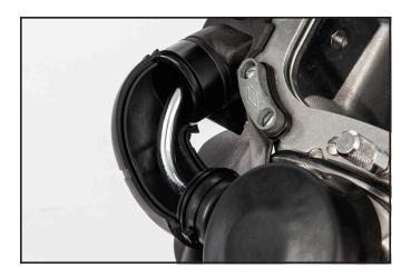
15) Line up the detail features of water tubes A & B, with the mating details of both adapter sleeves.
