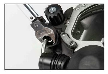
13) Line up the bent tube mount nut to the side block. Complete installation of bent tube assembly. Refer to "1.2.3 Installation of the Bent Tube Assembly" on page BNT-2 from the KMDSI modular manual.
