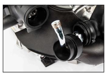
12) Swing the bent tube away from the side block and put the adapter sleeve (short), P/N 550-572, onto the bent tube assembly first, channeled end facing away from regulator inlet.
