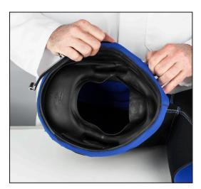
1. Reinstall the top and bottom bands into the new hood and face seal assembly P/N 510-710.
