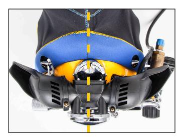
5. Using a torque screwdriver with a large Phillips attachment, torque the band screws to 26 inch pounds\* (2.94 Newton Meters).
