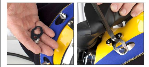
1. Remove the band keepers P/N 540-175 and 540-179.
