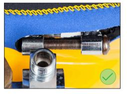
Make certain the bands are over the rubber of the molded face seal and the neoprene has NOT folded over the rubber.
