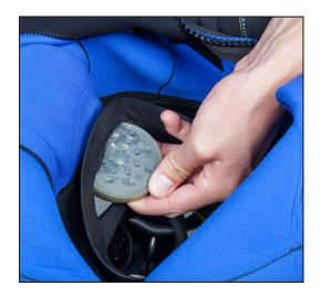
If the optional step to move the port whisker wing was followed, untuck the whisker wing, reinstall the screws, spacers and zinc whisker anode or kidney plate and torque the screws to 12 inch pounds (1.3 Newton Meters).
